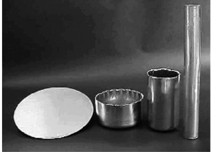
Fig. 8: Platinum alloy disc cut from sheet and cupped.
