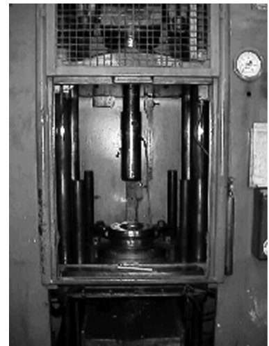
Fig. 9: Press used for cupping operations.
