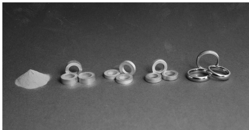
Fig. 1: Gold powder and rings at various stages of manufacture
