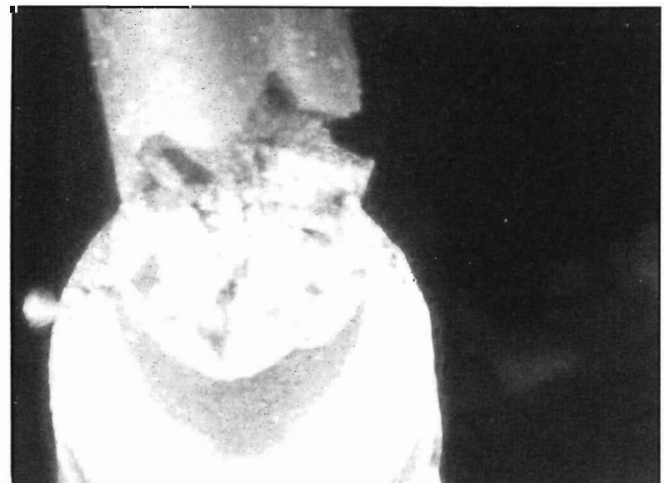
Figure 2. An embrittled cast article. Grain boundary fracture indicates loss of ductility.
