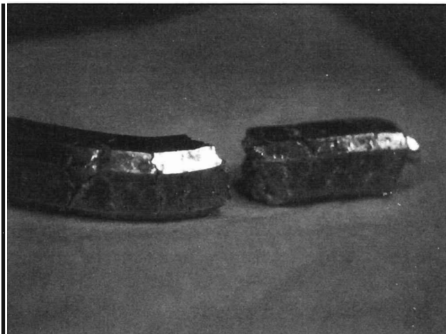
Figure 1. Overview of embrittled platinum with trace contamination that has destroyed physical properties for further working.
