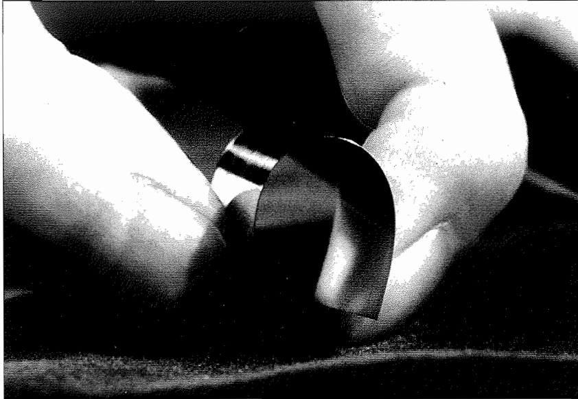
Platinum sheet manufactured using electroforming process.
